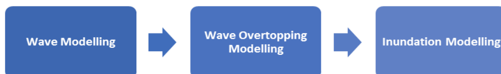
Figure 2-2: Modelling components of the wave overtopping assessment.
